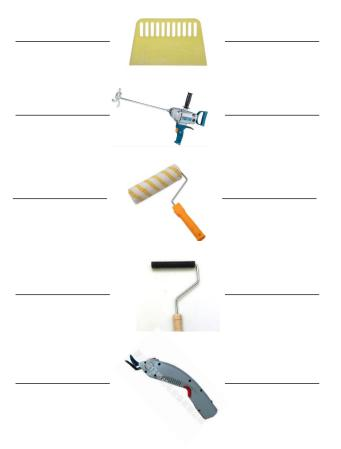
Plastic scraper: used for smooth the uneven carbon fiber sheet
