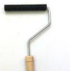
Thread roller: used for eliminating the bubbles of epoxy resin after pasting on the carbon fiber sheet
